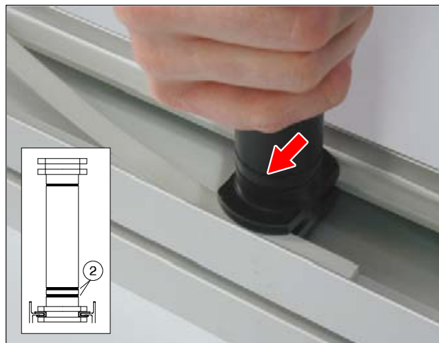
Fig. 16: Assembly mandrel - Installing the 2nd sliding strip
