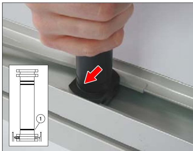
Fig. 15: Assembly mandrel - Installing the 1st sliding strip
