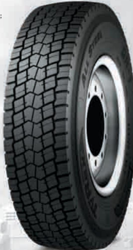
DR-1DR-1 model is intended for mounting on the driving axle of long-haul tractors MAN, VOLVO, Scania, MAZ, KAMAZ and buses.
