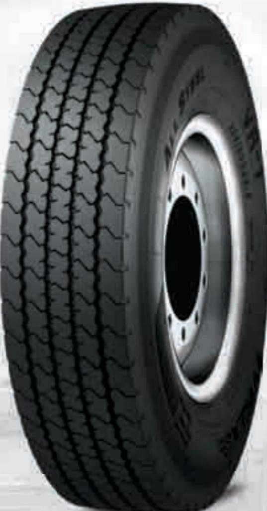
Truck tubeless radial All-Steel tyre intended for application on the steering and driving axles of busses. Introduction of new compound formulas for tread ply and improved tyre section provide better abrasive wear resistance, reduction of heat build-up and therefore lower rolling resistance.
