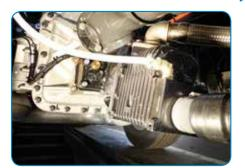
PF Option – PTO Flange Splined shaft for direct flange mounting on PTO
