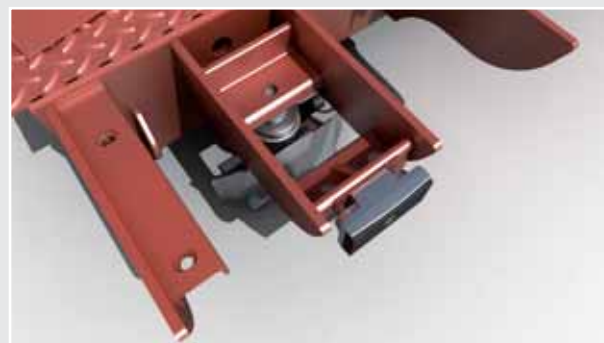
Double front edge complete with impact resistant buffers - extremely important to prevent deterioration of concrete in areas of contact while a vehicle is braking.
