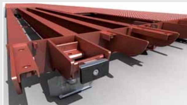
Longitudinal hatch supporting structure specially sized to optimise deck strength and system accuracy, even in harsh operating conditions. Sandblasting and subsequent painting of all the metallic parts to protect against oxidation. Special wax coating applied to all underside surfaces for optimum protection.
