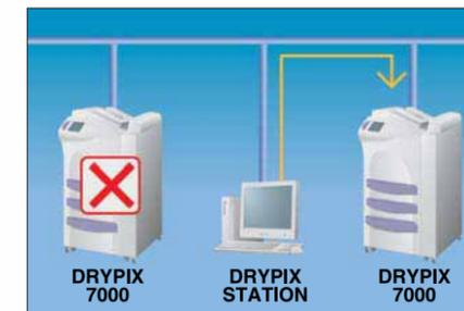
Optionally available DRYPIX STATION assures system reliability in multi-unit environments by automatically detecting printer failure and rerouting images to an active printer.
