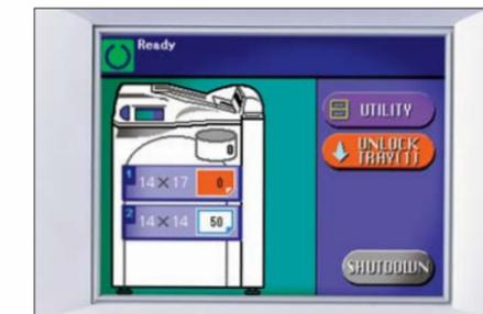
DRYPIX 7000’s newly developed touch-panel operation screen with icon-based interface simplifies operation and reduces operator error. All operations, from film loading to processing, can be carried out in daylight room conditions.
