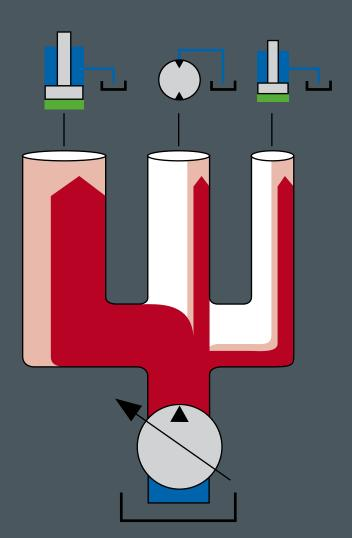
When operating several actuators at the same time, the available oil is divided according to the requirements of these functions. If all functions actuated together demand a higher flow than can be provided by the pump, the system is saturated. In this case all actuator flows will be reduced evenly. The ratio of their flows to each other remains the same, no actuator will stop unexpectedly. Besides the simplicity of operation, this also has advantages regarding safety.
