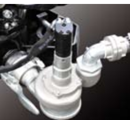
Drilling fluid suction pump.
