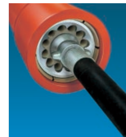
The ramming machine doesn't need the usual thread connection.
