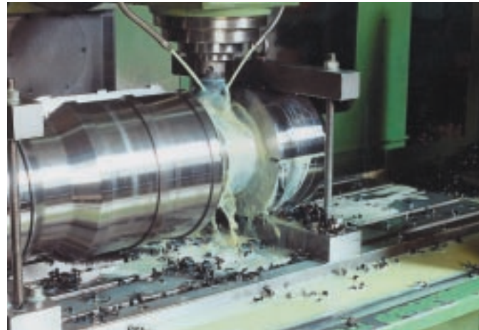
Having a tolerance of only 0.05 mm, the clamped work piece can be milled and drilled with extreme precision.
