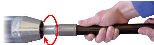
From GRUNDOMAT types 45 to 110 - Thrust control stud (Switch over with a 1/4 turn of the air hose)
