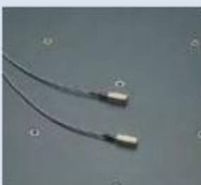
Temperature compensation system (photo : temperature sensors)
