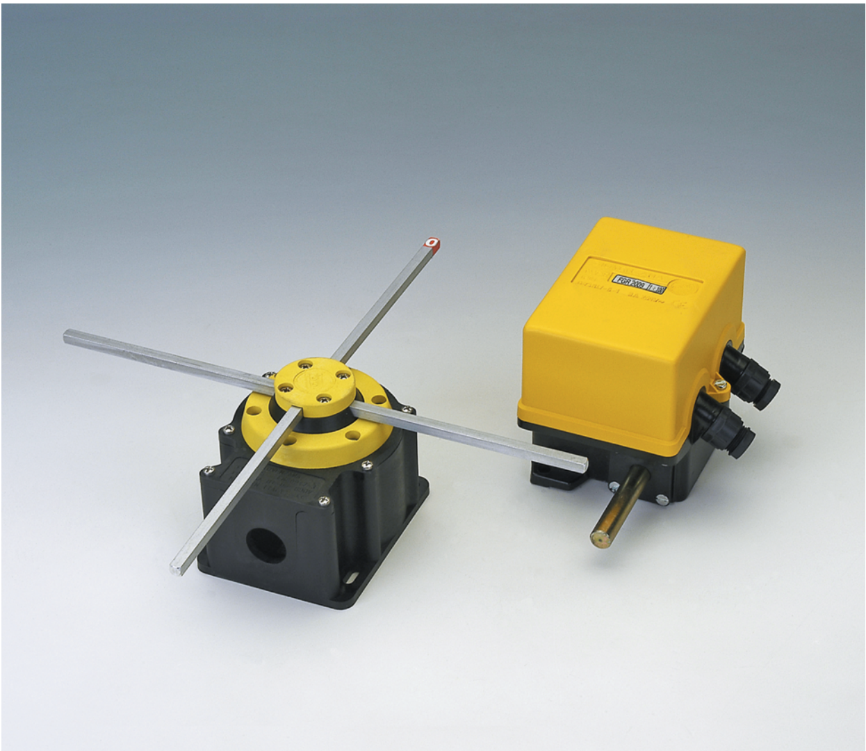
Rotary control switches with 300mm rods from 3 up to 5 positions. Control switches with rotary gear from 12 up to 200 rpm with 4 or 6 micro switches.
