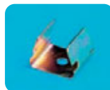
Fire Clip FCLIP Secures 2 x 1.5mm 2c Fire Performance cables to comply with BS5839pt1 use with metallic fixings
