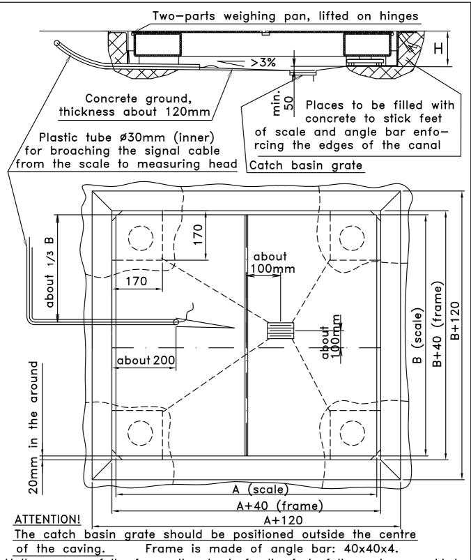
At the corners of the frame, the stands for the feet of the scale are welded.
