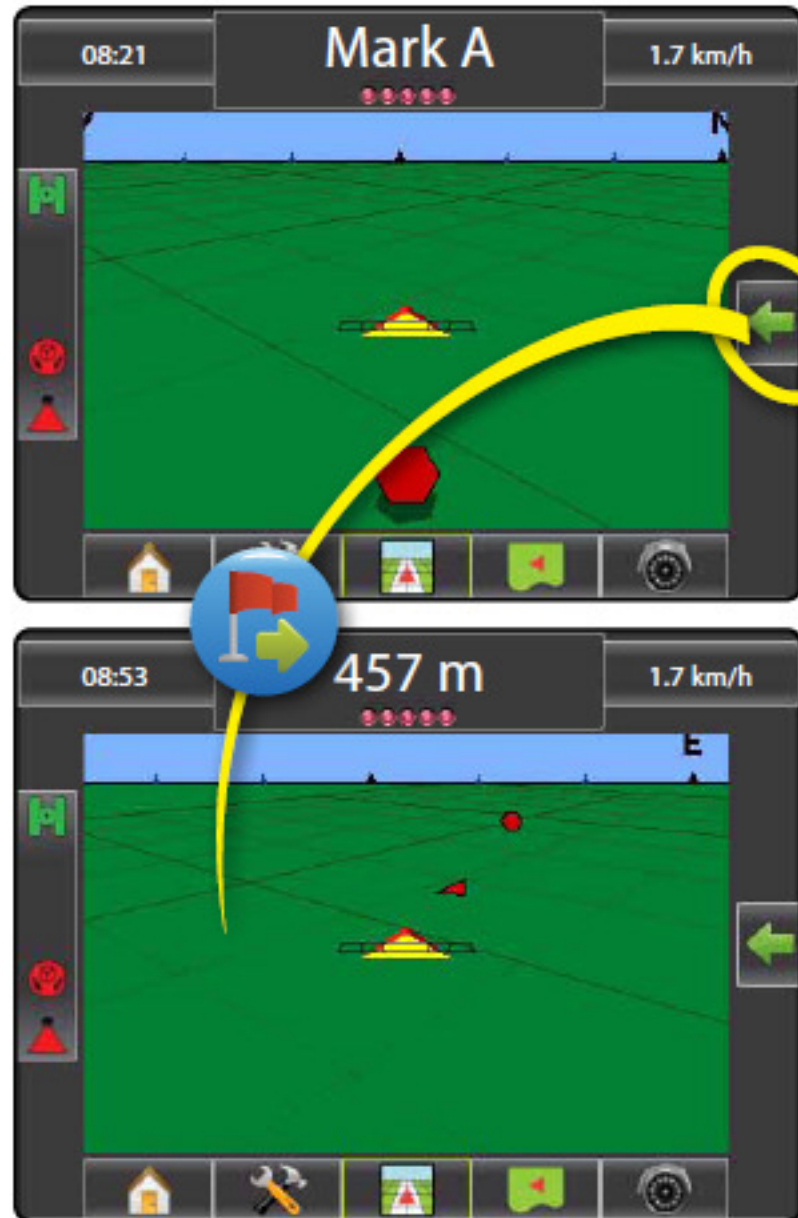
Figure 1-12: Return Point Established - Vehicle View
