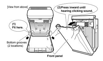
To correctly restore the front panel, press the front panel until hearing the clicking sound from the left and right sides.
