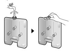
Close the water tank cap tightly. Unless tight, water may leak.
