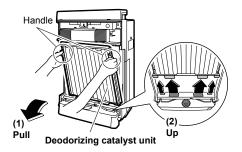
Replace the pleated filter with a new filter.
