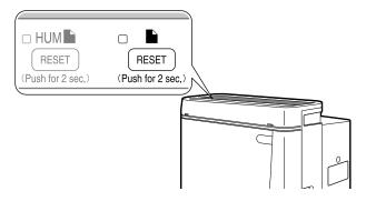
· After replacing the pleated filter, the Air-purifying filter lamp does not go out unless the filter reset button is pressed and held for 2 seconds.
