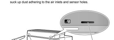
• Using a vacuum cleaner nozzle attachment with a narrow opening,
