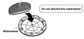
Tuck the humidifying filter underneath the tabs (6 locations) on the waterwheel so that it does not stick out from the waterwheel.
