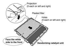
· Insert the pleated filter underneath the tabs (4 locations) at the top and bottom of the deodorizing catalyst unit.
