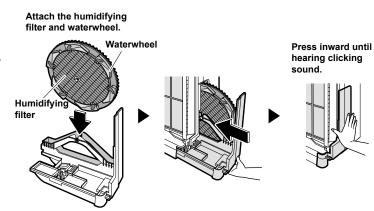
Install the humidifying filter and waterwheel in the direction shown in the figure.
