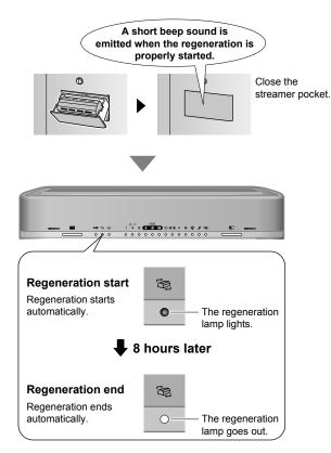
After regeneration ends, remove the recyclable deodorizing cartridge and return it to its place of use.
