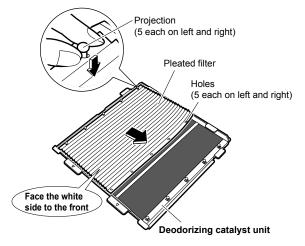
• Insert the pleated filter underneath the tabs (4 locations) at the top and bottom of the deodorizing catalyst unit.
