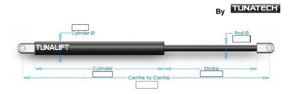
Gas springs provide a number of benefits in automotive, marine, industrial and domestic springing applications, especially wherever controlled damping is required. Whether displaced in tension or compression, gas springs provide a nearly constant force through their entire stroke as compared to coil or leaf metallic or composite springs. They can also be constructed with special features such as variable damping and blocking.
