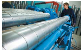
Spiral air ducts workshop
