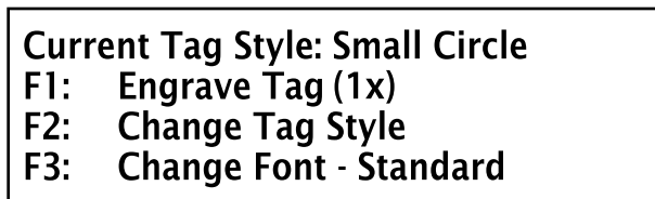
Fig. 4-4 When the tag is properly seated and the following screen is displayed, press “F1” to engrave an ID tag.
