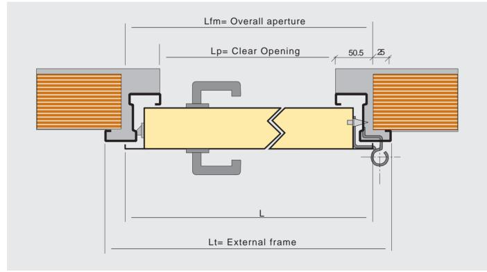
\* NOTE: The tolerance is<sub>+2</sub> mm for single leaf frames and  $^{-0}_{+3}$  mm for double leaf frames in cement/blockwork. For installation into a pre frame a tolerance of  $^{-0}_{+4}$ mm each side is necessary.
