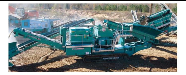
The Powerscreen range of mobile cone crushers are suitable for secondary and tertiary crushing in direct feed applications. The range uses advanced crusher technology to provide high volumes of excellently shaped product.
