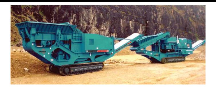
The Powerscreen® Pegson 1180 Premiertrak is a medium to large scale mobile primary jaw crusher plant that acheives high outputs in a variety of quarrying, recycling and contract crushing applications. The crusher features a high swing jaw with a forceful motion that improves feed entry into the crushing chamber to maximise throughput and allow for excellent reduction. User benefits include a low fuel consumption, track mobility and simplified set-up, operation and maintenance.
