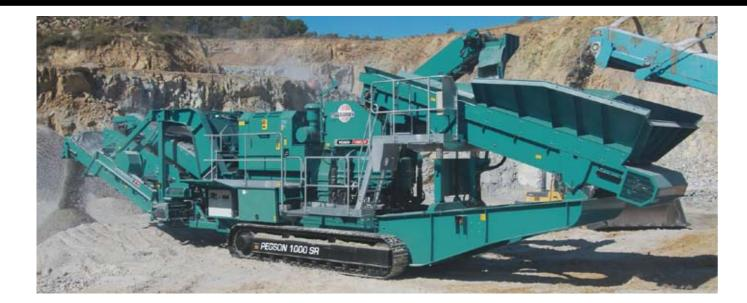
The high performance Powerscreen® Pegson 1000 Maxtrak is a small to medium sized cone crusher which has been designed for direct feed applications without pre-screening on clean rock. At its heart is the Automax® cone crusher which provides excellent reduction and product cubicity for the production of high quality aggregate and sub-base material. Hydraulic release capabilities are designed so that any uncrushable material entering the chamber is safely discharged.
