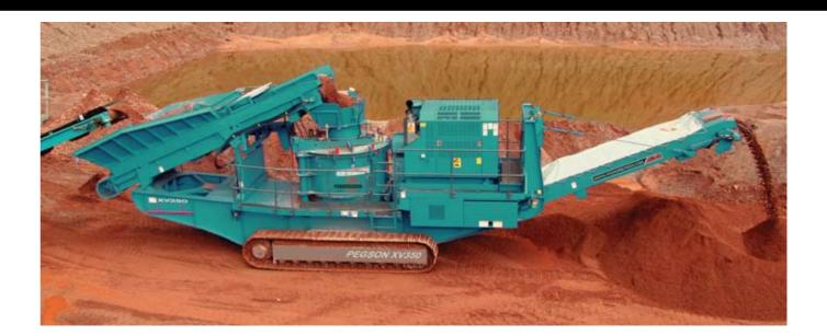
Powerscreen offer a range of mobile impact crushers suitable for primary and secondary applications including crushing aggregate, reinforced concrete and asphalt. The range includes both horizontal shaft impactors and vertical shaft impactors, both of which are designed to achieve a high ratio of product reduction.
