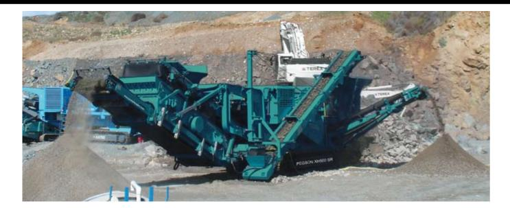
The Powerscreen® Pegson XH500 is the flagship horizontal shaft impactor. It is versatile, efficient and highly productive with an output potential of up to 500 tph. The Pegson XH500 offers both excellent reduction and a high consistency of product yield in quarrying, recycling and demolition applications. It is ideally suited to contract crushing due to its high productivity and ease of set-up, operation and maintenance.
