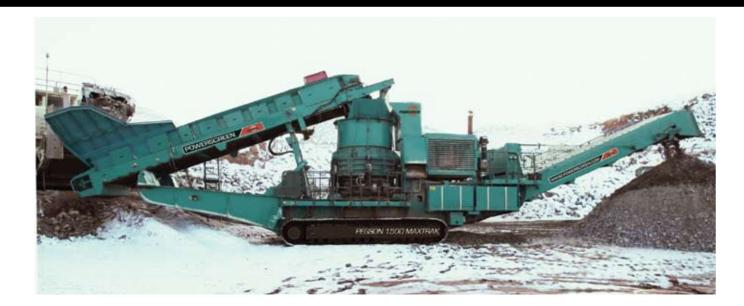
The Powerscreen® Pegson 1500 Maxtrak is one of the largest track mobile cone crushers on the market. Specifically developed for larger end users the plant can accept an "all in-feed" from a primary crusher to produce large volumes of aggregate.
