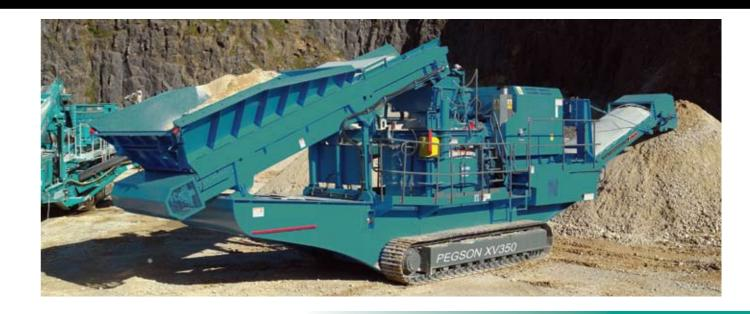
The Powerscreen® Pegson XV350 vertical shaft impactor has been designed for users who require a plant that excels at producing high specification, shaped product. With a range of crushing configurations available, the Pegson XV350 is versatile, productive and suitable for a number of applications including road building, concrete manufacture, manufactured sand, slag, and glass recycling.
