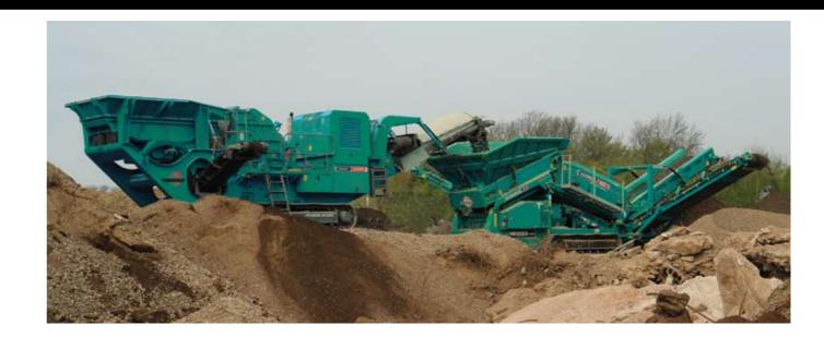
The Powerscreen® Pegson XH320 is a compact horizontal impact crusher designed to offer mid-sized operators and contractors both excellent reduction and high consistency of product shape for performance in quarry and recycling applications. With track mobility the plant is capable of working in the most demanding environments and features a rapid set-up time, fuel efficient direct drive system and excellent output potential.
