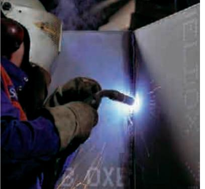
Welding. You can weld WELDOX together with all other types of steel, and use all common welding methods and consumables. To increase assurance against cold cracking, however, you may need to preheat the material. The preheating temperature doesn't need to be as high as when welding with other high-strength steels because WELDOX has lower content of alloy elements.
