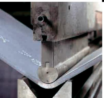
**Bending.** Because WELDOX is stronger than ordinary steel, more force per millimetre of plate thickness is required to bend the material. But thanks to WELDOX being stronger, the plate doesn't need to be as thick. This means that in practice, the requisite bending force is often lower.
