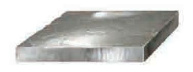
Improved flatness. Weldox has exceptionally good flatness, with the groundwork laid when the plate is rolled. Additionally, SSAB Oxelösund's quenching plant is designed to distribute cooling water evenly over the entire surface of the plate. This lets the plate cool more evenly and retain its flatness throughout the entire hardening process. Together, these processes combine to make Weldox flatter than competing plate.
