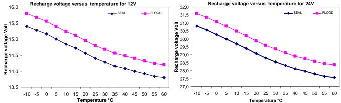
Fig. 6 Compensation curve of V<sub>ch</sub> recharge voltage according to the battery temperature
