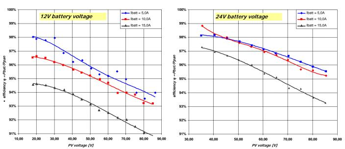
Fig. 7 WRM-15 efficiency versus voltage pannel for 12V e 24V battery.
