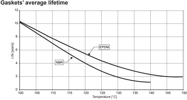
The diagram shows the indicative average lifetime, expressed in years, of the sealing gaskets based on the average temperature of the heating medium.
