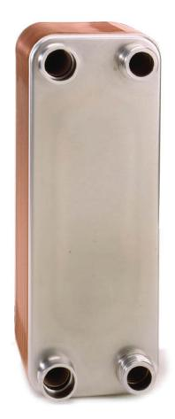
holes in each plate form four inlet and collection headers for the fluids, which are taken out through four passages on the surface of the front end plate. Braze welding is done around the edge of the plates and in the contact points between the V-shaped corrugations of the plates overlapping in an alternate way.
