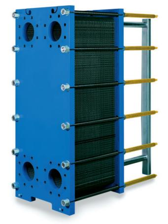
plates touch, forming very close and fragmentary inter-channels, and making the motion of the fluids extremely turbulent. Thanks to the perfect alignment of the packaged plates, the four holes in each plate form four inlet and collection headers for the fluids which are taken out through four passages (threaded stainless steel nozzles or flanged fittings) on the surface of the front frame plate. The materials used for the construction of the heat exchangers are:
