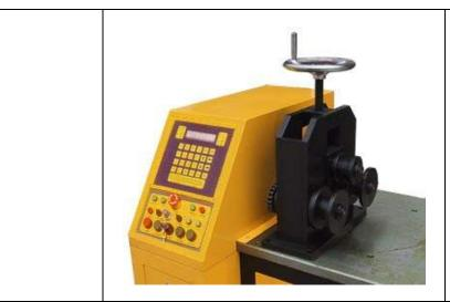
5. Arc-bending unit: All types of tube can be bent to the arc form. The finished arc shape bars are used to make gate frame, balcony, railing and stairs handrail. 1 mould (30mm width) accompanies with this unit
