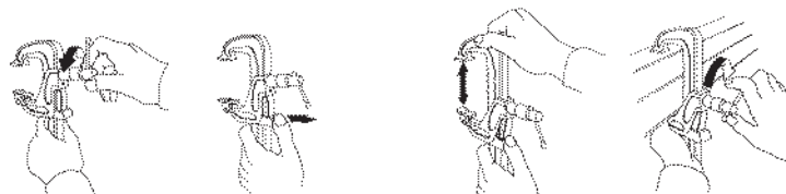
1. Loosen Screw 2. Push In Jaw Base 3. Slide Jaw Up or Down 4. Tighten Screw
