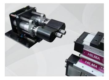
A single screw system to actuate the clamping areas is installed in the vicinity of the machining centre. The linear stroke of the screw system is actuated by a pneumatic cylinder. All positions are monitored via limit switches. The screw system automatically finds its position on the spindle of the clamping system.
