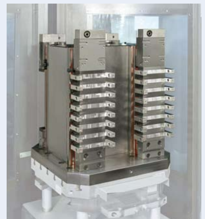
VL 125 Varioline with floating central jaws for multiple clamping
