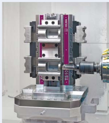
TS 125 tower clamping system with reversible step jaws
