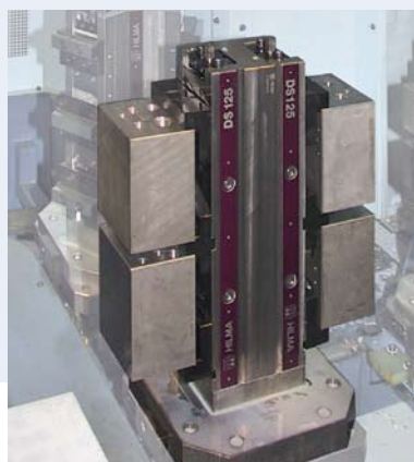
DS 125 double clamping system back-to-back, customer-specific
