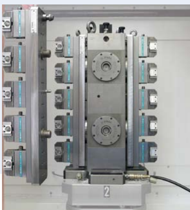
Clamping tower with zero-point clamping system and change plates with MC 40 Z
