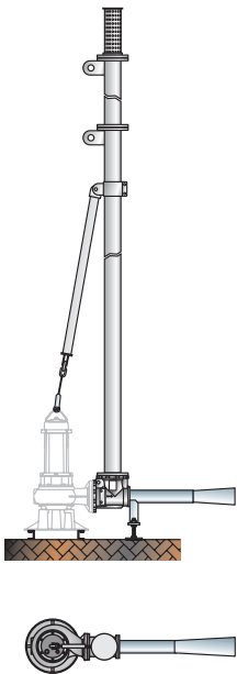
80/100 Ø OXY55/63 mm Ø diaphragm DN 80/100 ejector body 100 Ø air intake pipe
