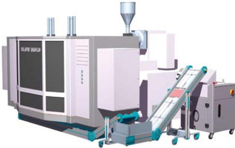
The drawing below shows the Plate Metal Detector inserted inside an N-CPR conveyor to detect metallic impurities when the material is being conveyed from the moulding unit to the recovery granulator.
