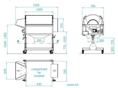
The SR – SM rotary drum separators are the most functional means for separating the product from the sprue.
