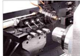
JSL-26AB / JSL-32AB The main spindle and sub-spindle perform machining synchronously.
