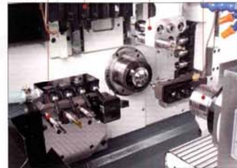
TOOLING SYSTEM External tool holder : 6 pcs Inner tool holder : 5 pcs Side drilling device : 5 pcs (JSL-26AB, 32AB) End drilling device : 4 pcs (JSL-26AB, 32AB)
