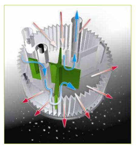
The suction power of the PLANEX SRM 45 E remains constant even when large amounts of dust are extracted:
