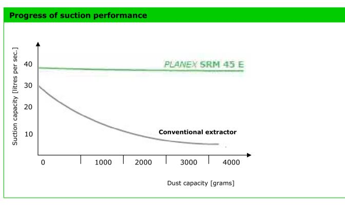
The automatic filter cleaning system keeps the suction power at a constant level.
