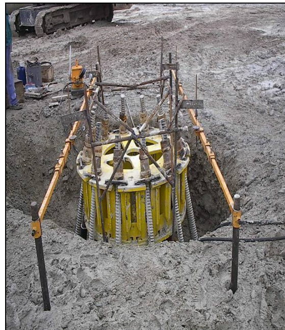
Compression load tests on piles with loads up to 14 000KN
