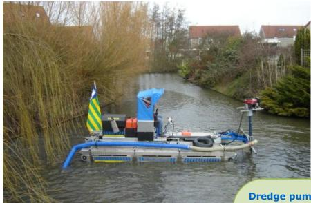
**Dredge pump** for sediment pumping.
