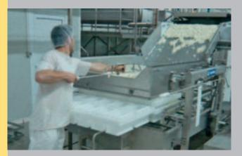
Effective and weightaccurate curd filling with the ALPMA filling unit type AFE.
