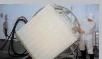
Low-budget startup equipment: Drainage of the cheese in stacks on the bottom floor with manual stack turning.
