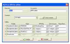
Energy Save solution is created with MR4-DP equipment, according to the area / floor car occupation. The system is able to activate/deactivate the electrical lines according with number of cars at the parking.
