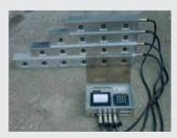
up to 5 sensor units, each installed in a robust aluminum housing, each equipped with ultrasonic sensors and laser sensors
