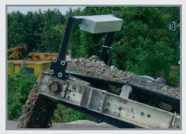
The sensors are contained in a robust, 100% dust-proof aluminum housing with a stable framework which can be mounted on the support frame of any conveyor belt.
