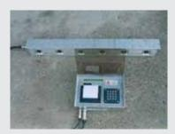
1 sensor unit installed in a robust aluminum housing, equipped with ultrasonic sensors and laser sensors
