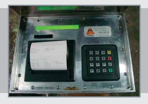
The processor unit is also the operational and system interface; the keypad and LCD display allow the user to set and check system parameters by simple menu navigation. The entire evaluation unit is enclosed in a 100% sealed aluminum housing.
