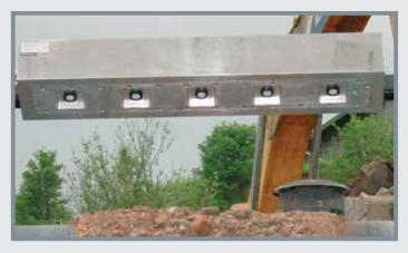
The sensor unit contains height sensors and path sensors which serve to collect data.
