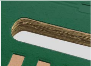
Cutting of mounting holes
