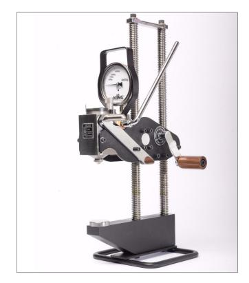
The test conditions and accuracy meet the requirements of ISO 6056 and ASTM E110 and can be used to test rough castings, forgings, nonferrous metals and semi-finished products after heat treatment. The result is far more accurate and repeatable than other portable Brinell hardness testers. The calibrated accuracy of the test force is 1% which confirms to ASTM E10.
