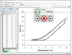
Control of the test stand using SAUTER PC software  $\ensuremath{\mathsf{AFH}}$
