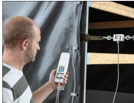
Universal digital force gauge for tensile and compressive force measurements with external measuring cell
