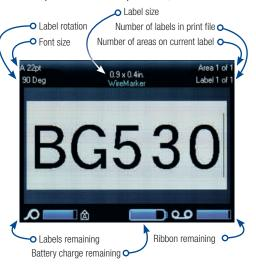
Every BMP61 label and ribbon is automatically recognised and auto-calibrated by the printer. The printer's colour touch screen displays which label material is currently installed and how many labels, how much ink and how much battery is left for maximum ease of use.
