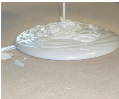
*Mapefloor Decor 700 poured on the substrate immediately after mixing*
