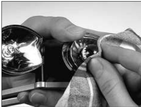
Fig. 51 Replacing the front direction indicator bulb
