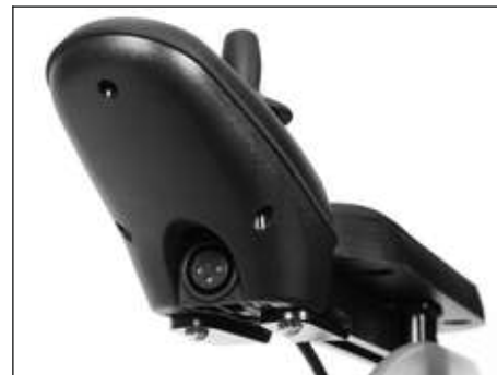
Fig. 19 Charging / programming receptacle on the control panel
