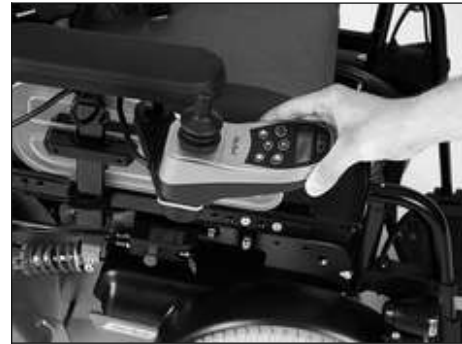
Fig. 34 Swing-away control panel holder with removable control panel
