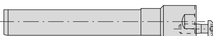
Serrated tool bodies in tool steel Corps crantés en acier rapide Ø .787" – 1.339" (Ø 20 – 34 mm)
