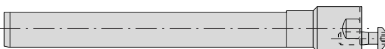
Serrated tool bodies in carbide Corps crantés en métal dur Ø .787" – 1.339" (Ø 20 – 34 mm)
