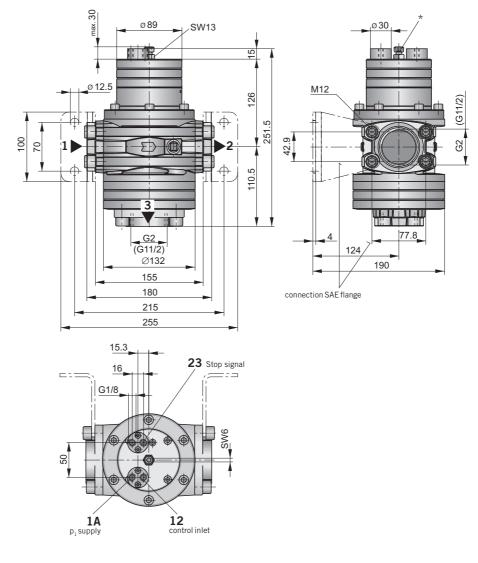
\* Adjusting screw for start time selection (socket head screw SW 6)
