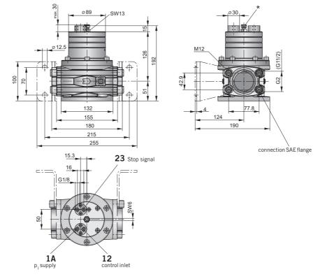
\* Adjusting screw for start time selection (socket head screw SW 6)
