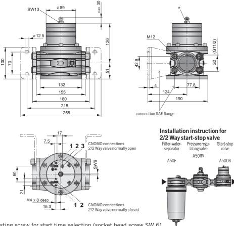
\* Adjusting screw for start time selection (socket head screw SW 6)
