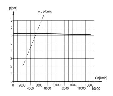
Pressure regulating valve – pilot operated Type: A50R-11/2, -2 Type: A50RV-11/2, -2
