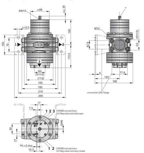
\* Adjusting screw for start time selection (socket head screw SW 6)
