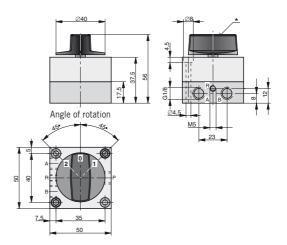
\* After removing the cover and loosening the mounting screws, the rotary switch is infinitely variable.
