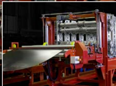
The sheet entry table is hydraulically ascending and descending. The upper-level-sheet-entry can also be conveniently done at normal working height.
