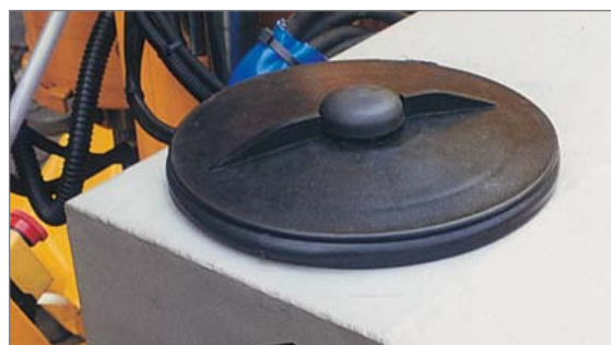
water filling opening
