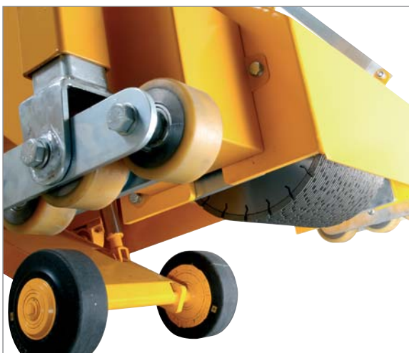
milling shaft of the CF-245 with a milling width up to 400 mm, height-adjustable and lockable block of support rolls for exact milling depth adjustment
